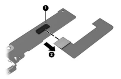
6. Remove the WLAN ribbon cable.
